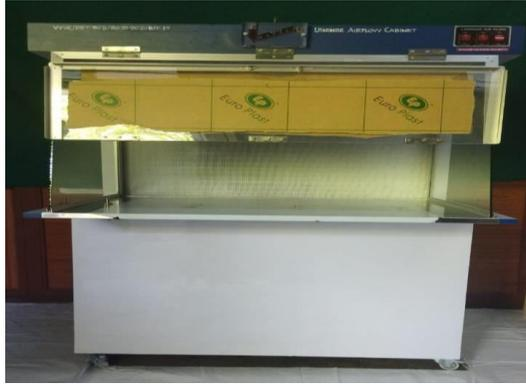
Laminar Air flow chamber is used to transfer the microbial culture in aseptic condition. This equipment is used for providing an excellent aseptic worktable for processes like sub-culturing, inoculation, assays sterile drug preparation etc.,
