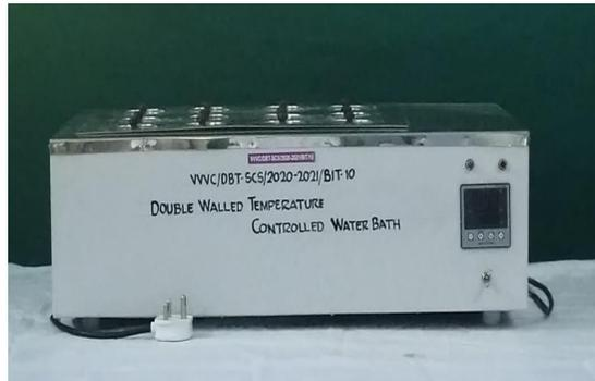
Thermostatic water bath is used for incubation of test samples underwater at constant temperature over a long period of time.
