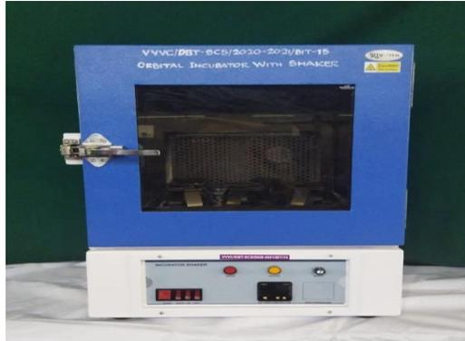
Incubator shaker is a temperature controlled instrument which is carried out both incubation and shaking functions, used in cell culture, fermentation, hybridization under controlled temperature and shaking speed.
