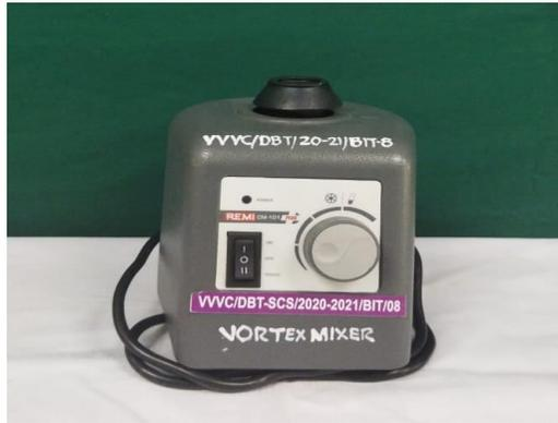
The vortex mixer is a bench top vibrator designed to operate with direct ON and Speed control option. The instrument is designed for vortex mixing of liquids in laboratories, school or factories.
