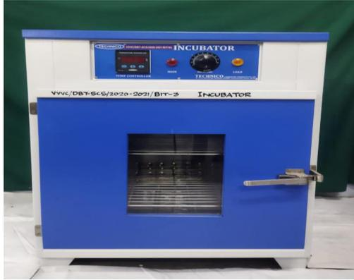
Incubator is a device which provides and maintains all artificial optimal conditions for growth of microbial culture.
