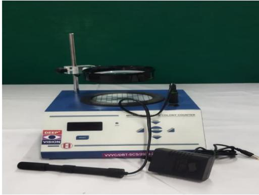
Colony counter is an instrument, used to count microbial colonies on a agar plate containing a growth medium.
