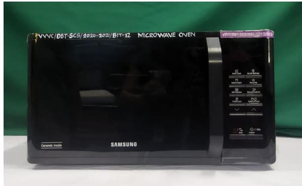
Microwaves are high frequency electromagnetic waves the energy released enable the microbiological media to be heated without changing either the form or the colour. Microwaves generated by the magnetron reflected at cavity and are distributed uniformly as the media rotates on the turntable.
