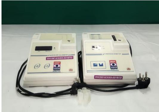
Photo colorimeter measures the intensity of colour concentration of any substance in the solution. The intensity of colour of a substance is in direct proportion to its concentration which in turn is measured in terms of transmittance / optical density.
