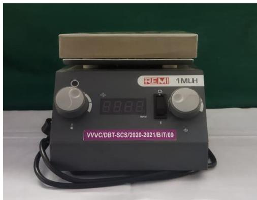
A hot plate magnetic stirrer is used for mixing and heating aqueous solutions simultaneously to speed up the reaction and dissolve the solute in the solvent.
