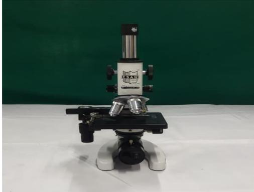
The Light Microscope enables us to view things that are too small to be seen with the naked eye. It uses a system of two or more lenses to collect and focus the transmitted visible light through a specimen to the eye. Animal cells, plant cells, protozoa and bacteria can be easily seen
