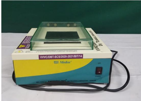
Transilluminator is used to study the results of electrophoretic patterns accurately. Gels after staining are placed on transilluminator and image can be seen directly by naked eye.
