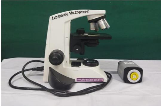
LCD Digital Microscope is an efficient tool to analyse various objects from micro-fabricated parts to large electronic devices. It can be connected to a TV or Projector for demonstration work.
